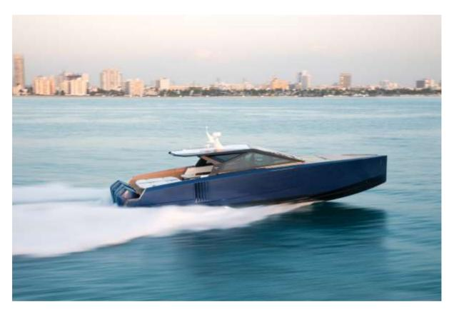
It is the first Wally yacht to be fitted with the new 600hp Mercury V12 Verado – or rather, a powerful configuration of four of them. With 2,400hp on the transom, the stable and efficient deep V-hull can reach an exhilarating 50 knots. And yet fuel consumption remains low, while the boat's additional tankage gives it a range of 300 nautical miles.
