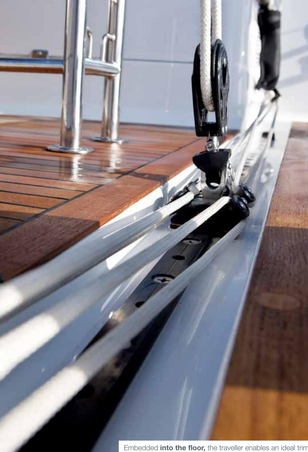
Embedded **into the floor**, the traveller enables an ideal trim.
