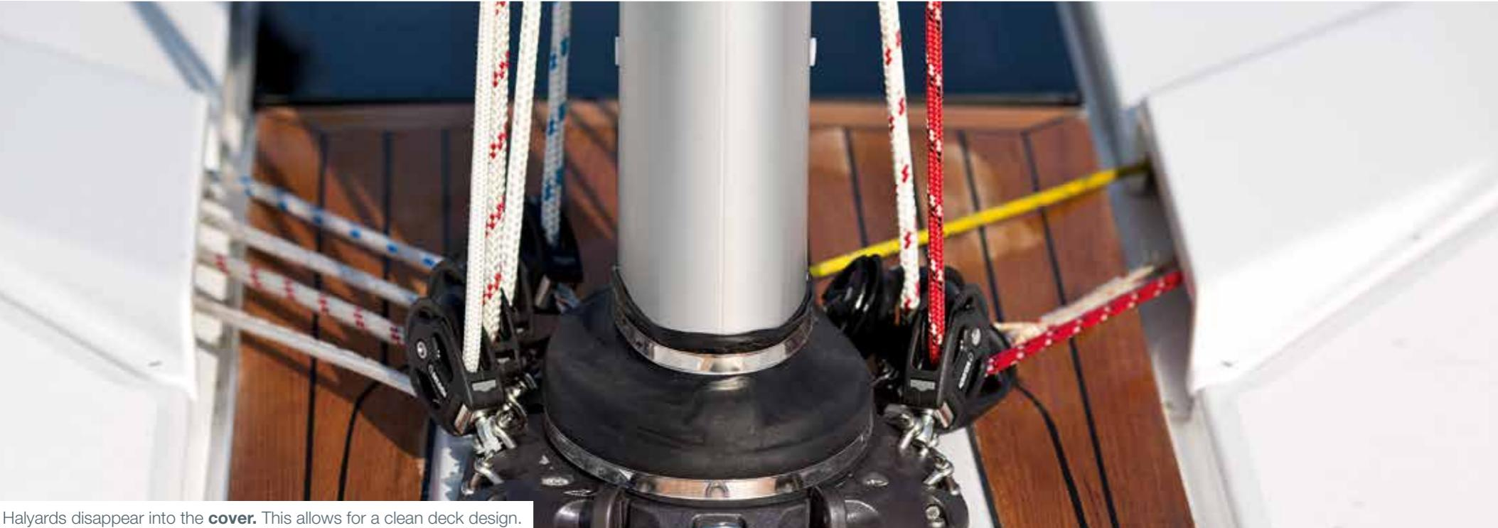
Halyards disappear into the **cover**. This allows for a clean deck design.
