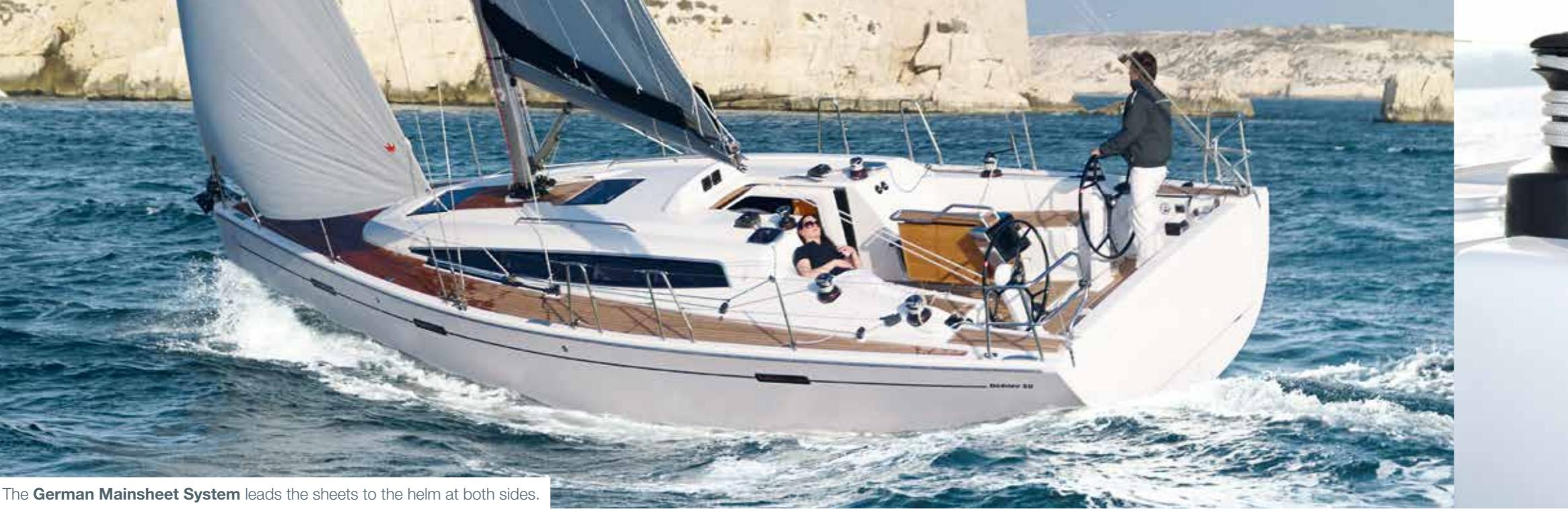
The **German Mainsheet System** leads the sheets to the helm at both sides.
